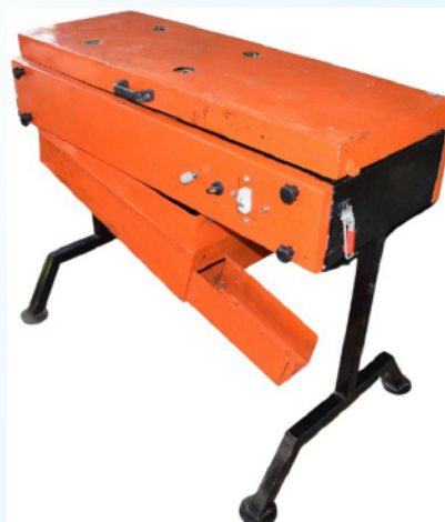
Fig. 7 View of portable semi-automatic cashew apple and nut separator
