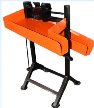
Fig. 6 View of portable pedal operated shear type cashew apple and nut separator
